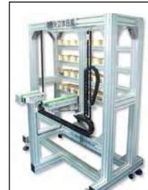
Small scale automatic storage system
