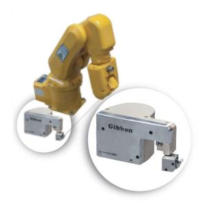
Gibbon Robot Quick Calibration System consists of dedicated measuring sensor and calibration software. It amends the parameters of robot's joint zero position, arm length, tool center point by simple and quick data collection process, increasing the absolute precision of robot effectively when working.
